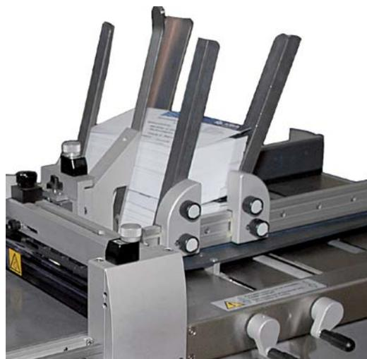
**Stack-to-stack processing enables orderly feed and removal of flat print materials.**
