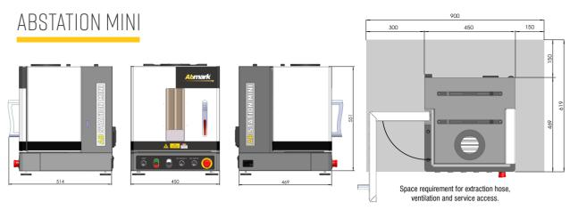
ABSTATION-MINI is a compact benchtop laser marking workstation that has been designed to be compatible with the full range of Abmark lasers. The workstation features a motorised Z-axis as standard with a base plate for attaching custom tooling.
